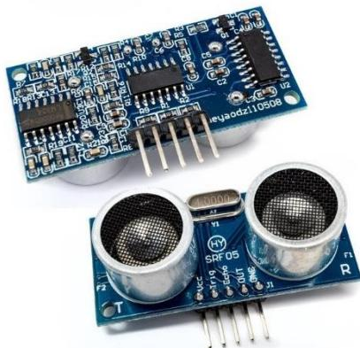
Fig. 33 Ultrasonic sensor [32]
